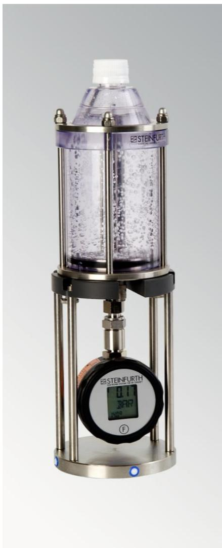
The Check Bottle TS 94.5 is used for monitoring the accuracy of the measuring heads of the CO<sub>2</sub> tester TS 91.7. It consists chiefly of a polycarbonate container and an integrated digital precision instrument, combining manometer and thermometer.
