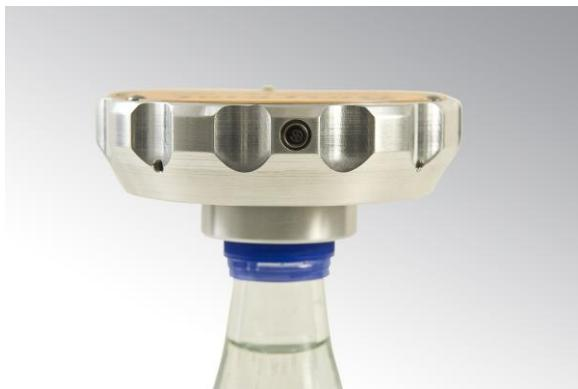
In the food & beverage industry, the opening torque of bottles and other containers with twist-off closures is an important quality parameter and vital for customer satisfaction.
