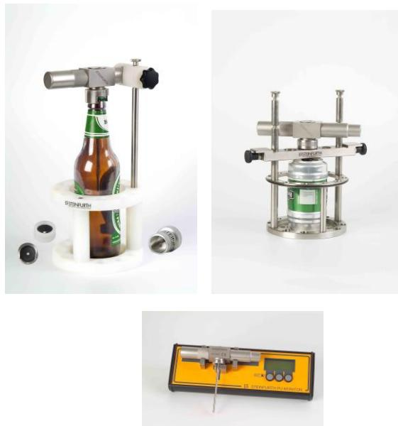
The Steinfurth PastControl system simplifies this task. The safe and simple operation requires only a short instruction to the operation personnel. The PU value can be read from the PU monitor's display directly at the pasteuriser line.
