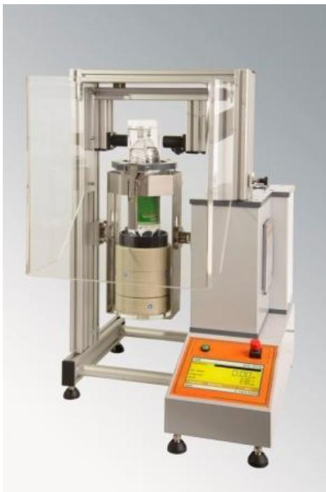
Lower precision and higher vulnerability of optical Co<sub>2</sub> measurement methods prohibit their primary use for analysis of carbon-dioxide packed beverages. The new OST (Steinfurth Optical Shelf Life Tester) combines the non destructive functionality of the optical measurement with another precise measuring method delivering on this way a new interesting application for this technology.
