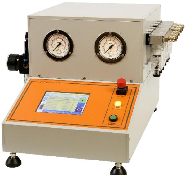
Package testing often requires defined pressure sequences. The IPPS can be programmed with up to 99 different pressure sequences. The programming can be done by the operator; special knowledge isn't necessary. Once programmed, the pressure sequences can be selected and activated. The duration of a sequence can vary from seconds to months. Repetitions are also possible.
