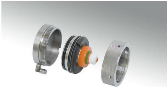
The PET bottle finish fixture is a means for pressure testing closures on finishes of existing PET bottles if a preform isn't available for that purpose. It is designed for use inside the safety tank of the Steinfurth Closure Tester V4. It is made entirely of stainless steel and other water-resistant materials.
