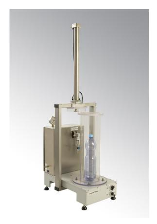
Resistance against interior pressure should be tested frequently, but at least when a new closure design is to be introduced. The Steinfurth Closure Tester gives you the opportunity to safely perform and observe this test under water in a stable plastic tank.
