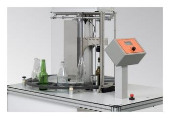
Routine sampling from beverage containers for analytical purposes may result in considerable strain for additional laboratory work. While sampling consists of a few simple movements, these have to be attentively performed and often every few minutes interrupt other tasks that require full concentration. Especially if great numbers of samples must be taken and the main analytical work is already semi-automated, manual operation of a sampling device poses an additional work time (= costs).
